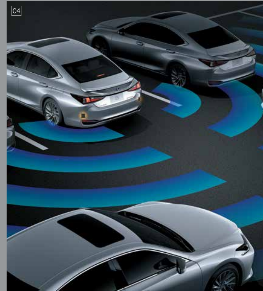
04 / Clearance Sonar The system detects static objects, such as a wall at the front and the rear of the vehicle. The driver is alerted by a buzzer and a display indicator showing the position relative to the static object and the level of danger in the center display and head up display.
